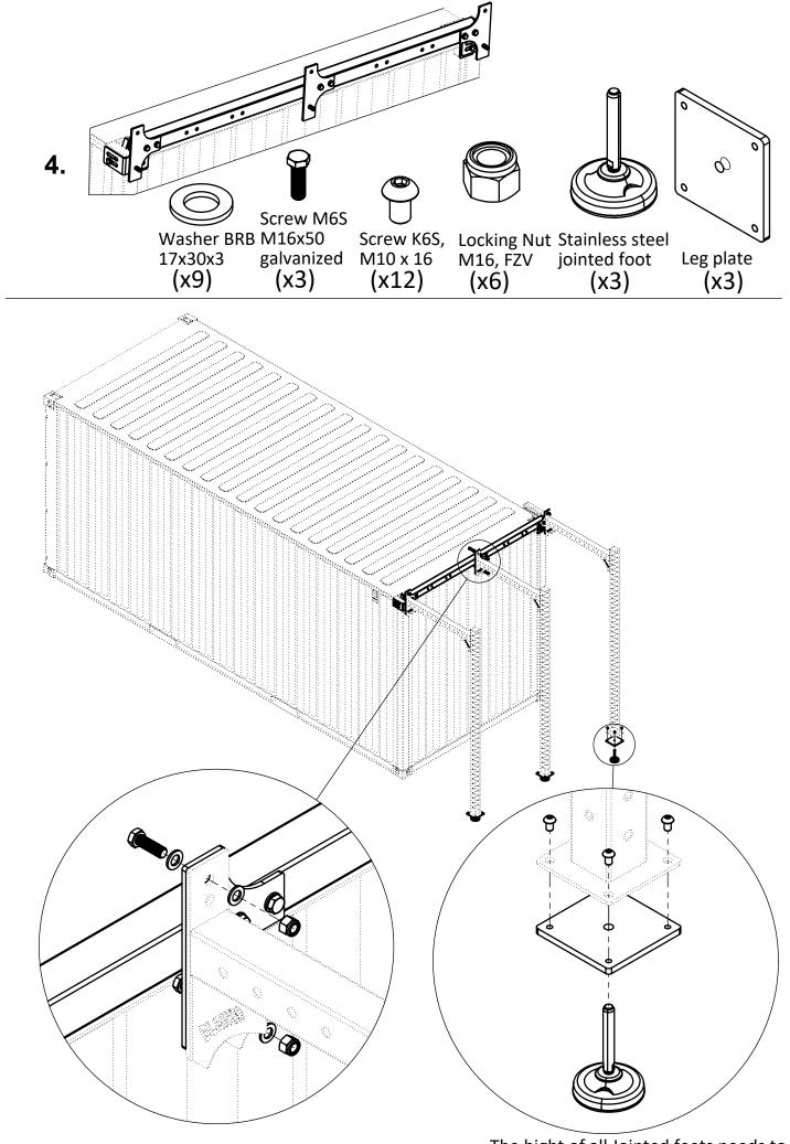
The hight of all Jointed feets needs to be adjusted according to ground level.
